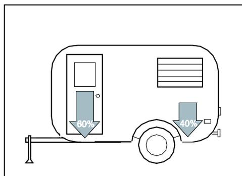
**⚠ WARNING-**The trailer load should be balanced equally from side-to-side. Unequal side-to-side loading can negatively affect handling and braking. Once in place, all cargo should be firmly secured to prevent shifting. If the load should shift abruptly during braking or cornering, it could adversely affect the handling of your vehicle and cause a very unsafe situation and may lead to an accident or personal injury.
