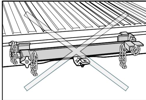
**Weight-Distributing Hitch System** – This type of system uses a "load-leveling" or "equalizing" hitch. The weight-distributing feature helps shift the trailer tongue weight to all the axles of the tow vehicle and the trailer axles.
