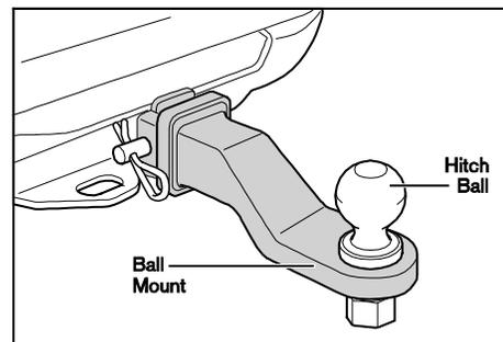
hitch ball in a 2" coupler, for example, could result in the trailer separating from the tow vehicle. The required hitch ball size is stamped on most trailer couplers.
