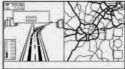
While driving on a freeway, when the vehicle approaches a junction, the system automatically switches to the split screen view and displays an enlarged view of the junction on the left side of the screen.
