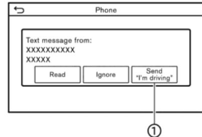
When the cellular phone connected to the vehicle receives a text message, a notification will appear on the upper display and on the vehicle information display with a tone.
