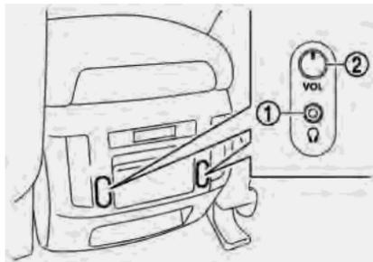
Commercially available headphones can also be used by connecting them to the headphone jacks ① located at the rear of the center console box.
