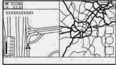
When approaching a guide point, the system automatically changes to the split screen view and shows an enlarged view of the intersection on the left side of the screen. The distance to the guide point and the name of the next street to drive on are displayed at the top of the screen.
