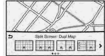
Push <MAP/VOICE> on the INFINITI controller (models with navigation system) while the current vehicle location is displayed on the map, or push <DISP> on the INFINITI controller (models without navigation system) to show the display view bar.
