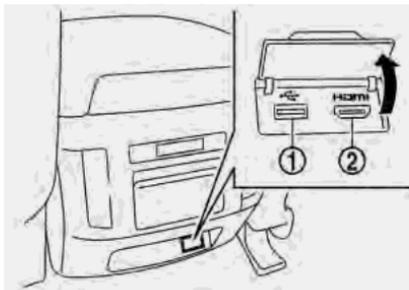
USB connection port ① and HDMI port ② are located at the rear of the center console box.
