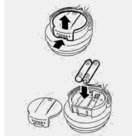
1. Open the lid as illustrated above. Use a flat object, such as a coin, if necessary, to open the lid located on the back of the left headphone speaker.
