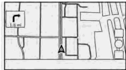
When route guidance starts, the small turn arrow and the distance to the next guide point are displayed in the upper left corner of the map screen. This arrow indicates the turning direction at the next guide point (corner or intersection). When approaching a guide point, an enlarged intersection view is displayed. Also, there may be cases where
