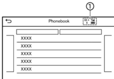
When a cellular phone is connected through the Bluetooth® wireless connection, indicators ① for phone and text messaging are displayed on the upper display.
