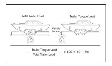
rearward of the trailer tongue and will not give you an accurate measurement of the true tongue load. Make sure the vehicle jack is placed directly under the trailer tongue coupler, and the tongue is set at the height/level of the tow vehicle hitch.
