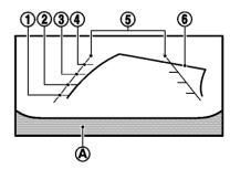
Guiding lines that indicate the vehicle width and distances to objects with reference to the bumper line (A) are displayed on the monitor.
