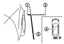
Guiding lines that indicate the width and the front end of the vehicle are displayed on the monitor.
