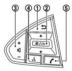
The steering-wheel switches mainly controls the upper display (adjust the volume, select a menu, voice recognition, Handsfree phone).
