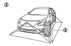
There are some areas where the system will not show objects and the system does not warn of moving objects. When in the front or the rear view display, an object below the bumper or on the ground may not be viewed ①. When in the bird's-eye view, a tall object near the seam ③ of the
