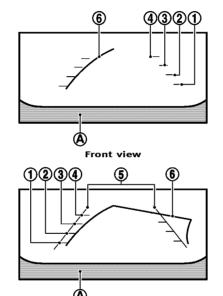
Guiding lines, which indicate the vehicle width and distances to objects with reference to the vehicle body line (A), are displayed on the monitor.
