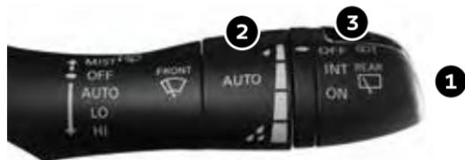
Move the lever (1) up or down to one of the following positions to operate the windshield wipers:
