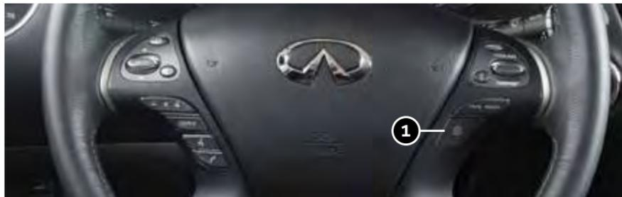
The Dynamic Driver Assistance switch ① can be used to temporarily turn on and off the following systems:
