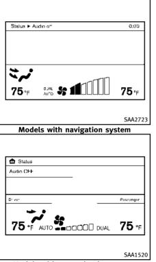
You can individually set the driver and front passenger side temperature using each temperature control button.
