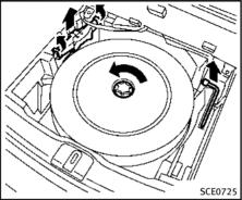
Remove jacking tools and the spare tire located under the luggage room as illustrated.
