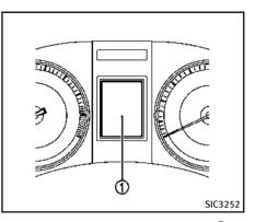
The dot matrix liquid crystal display ① is located between the tachometer and the speedometer, and it displays the automatic transmission position indicator, the Intelligent Cruise Control (ICC) system (if so equipped), the Distance Control Assist (DCA) system (if so equipped) information, the Intelligent Key operation information and other warnings and information.
