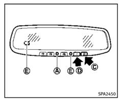
The indicator light will turn off. Push the "I" switch  $(\mathbf{D})$  to turn the system on.
