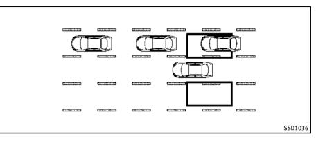
If the driver activates the turn signal while another vehicle is in the detection zone, then the BSW indicator light flashes and a chime will sound twice.
