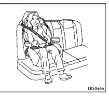
If the booster seat is compatible with your vehicle, place your child in the booster seat and check the various adjustments to be sure the booster seat is compatible with your child. Always follow all recommended procedures.
