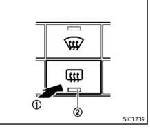
To defog/defrost the rear window glass and outside mirrors, start the engine and push the switch ① on. The indicator light ② will come on. Push the switch again to turn the defroster off.
