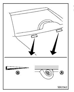
If you wax the surface of the hood, be careful not to let wax get into the washer nozzle (A). This may cause clogging or improper windshield washer operation. If wax gets into the nozzle, remove it with a needle or small pin (B). Be careful not to damage the nozzle.
