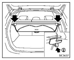
To stow the cargo cover, remove it from the hooks and hold until it is retracted. Make sure that the cargo cover is snapped into the holders (2) to keep it from moving around while driving.
