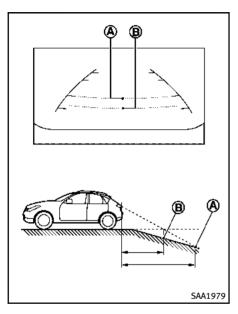
is the place  $(\mathbf{B})$ . Note that any object on the hill is closer than it appears on the monitor.
