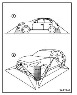
There are some areas where the system will not show objects. When in the front or the rearview display, an object below the bumper or on the ground may not be viewed (1). When in the bird-eye view, a tall object near the seam of the camera viewing areas will not appear in the monitor 2.
