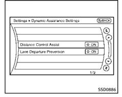
3. To set the DCA system to on or off, highlight the "Distance Control Assist" key, select ON or OFF and push the ENTER (2) button.
