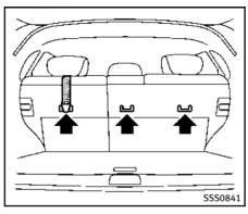
First, secure the child restraint with the LATCH lower anchors (rear outboard seating positions only) or the seat belt, as applicable.
