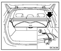
To remove the cargo cover, stow the cover and pull the holder to the opposite side ③.
