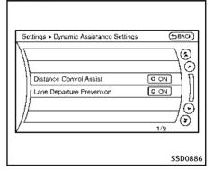
3. To set the LDP system to on or off, highlight the "Lane Departure Prevention" key, select ON or OFF and push the ENTER (2) button.
