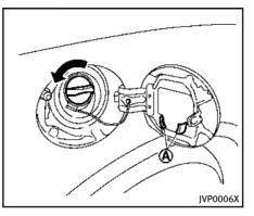
Turn the fuel-filler cap counterclockwise to remove. To tighten, turn the cap clockwise until a single click is heard.
