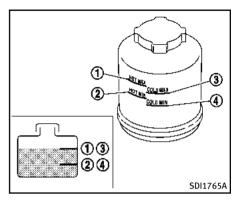
Check the fluid level in the reservoir.
