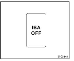
The vehicle should be driven with the Intelligent Brake Assist (IBA) system on for most driving conditions.
