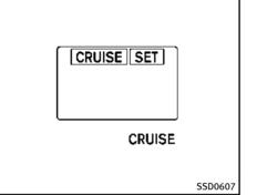
When the ignition switch is pushed to the ON position, the indicators come on as illustrated to check for a burned-out bulb, and it turns off when the engine is started.
