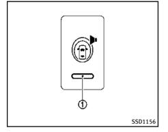
The warning systems switch will turn on and off the Lane Departure Warning (LDW) system, the Blind Spot Warning (BSW) system and the Forward Collision Warning (FCW) system at the same time.
