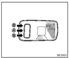
When the switch is in the DOOR position  $(\widehat{A})$ , the light illuminates while the lift gate is opened. When the lift gate is closed, the light will turn off.
