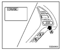
Operating conventional (fixed speed) cruise control mode To turn on the conventional (fixed speed) cruise control mode, push and hold the MAIN switch (A) for longer than about 1.5 seconds.
