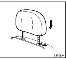
To lower, push and hold the lock knob and push the head restraint down.
