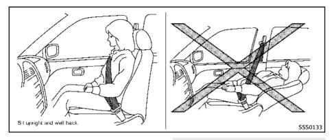
senger sits well back and straight up in the seat. If the seat back is reclined, the risk of sliding under the lap belt and being injured is increased.
