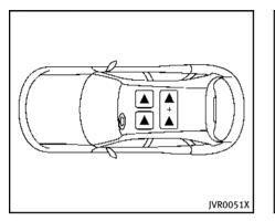
The illustration shows the seating positions equipped with head restraints and headrest. The head restraints are adjustable.
