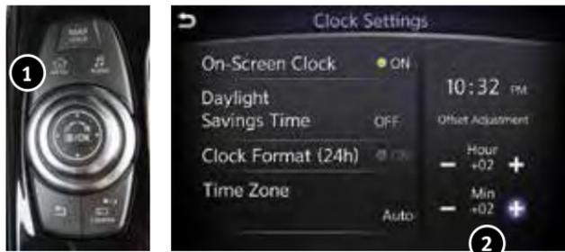
To adjust the time and the appearance of the clock on the display:
