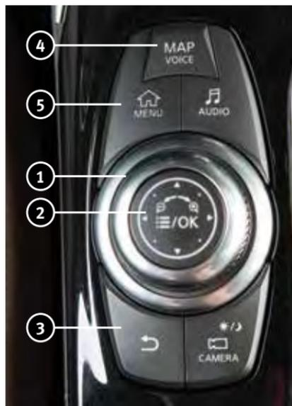
Use the Infiniti controller ① and **OK** button ② to navigate through the center display screens.
