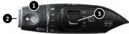
Turn the switch ① to one of the following positions to operate the windshield wipers:
