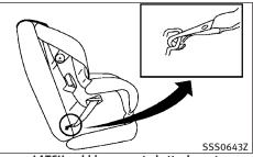
LATCH webbing-mounted attachment Installing child restraint LATCH lower anchor attachments
