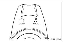
INFINITI controller AUDIO button Push **(AUDIO)** to display the current audio screen.
