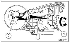
Low/High beam Headlight bulb replacement:
