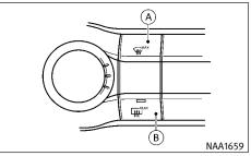
The defroster switch (B) operates when the ignition switch is in the ON position for the rear window, and (if equipped) for the outside rear view mirrors.
