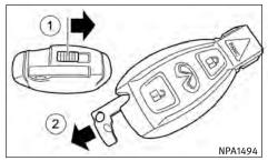
Push release catch (1) in the direction of the arrow and, at the same time, remove emergency key element (2) from the key.
