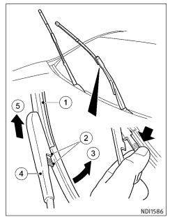
REPLACING FRONT WINDOW WIPER BLADES
