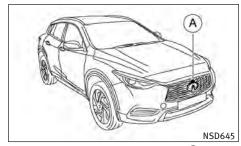
The FEB system uses a radar sensor (A) located behind the INFINITI logo to measure the distance to the vehicle ahead in the traveling lane.
