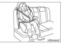
lower than the center of the child's ears, a high back booster seat (2) should be used.
