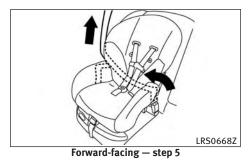
Allow the seat belt to retract. Pull up on the shoulder belt to remove any slack in the belt.
