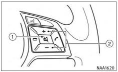
Steering wheel mounted audio control buttons
