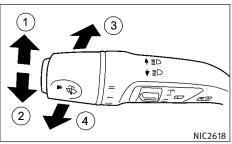
Switching High Beam Assist on/off
