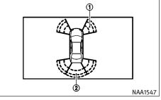
When the corner of the vehicle moves closer to an object, the corner sensor indicators (1) appear (if equipped).
