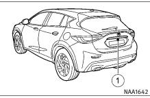
To display the rear view, the RearView Monitor system uses a camera located just above the vehicle's rear license plate (1).
