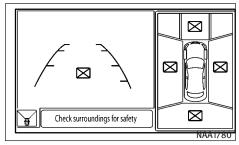
When the [X] icon is displayed on the screen, the camera image may be receiving temporary electronic disturbances from surrounding devices. This will not hinder normal driving operation but the system should be inspected. It is recommended you visit an INFINITI retailer for this service.
