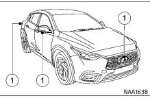
To display the multiple views, the Around View Monitor system uses cameras (1) located in the front grille, on the vehicle's outside mirrors and one just above the vehicle's rear number plate.
