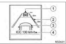
Display when the ICC system is activated
