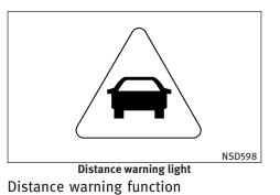
The distance warning function can help you to minimize the risk of a collision with the vehicle in front or reduce the effects of such a collision. If the distance warning function detects that there is a risk of a collision, you will be warned visually and audibly.
