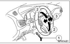
Release the lock lever ① as illustrated and adjust the steering wheel to the desired position (up or down ②, forwards or backwards ③). Firmly push the lock lever back into position to lock the steering wheel in place.
