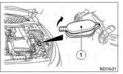
Fill the windshield-washer fluid reservoir periodically. Add fluid when the low washer fluid warning appears on the vehicle information display.
