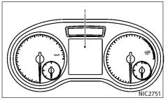
The vehicle information display (1) is located between the tachometer and the speedometer.
