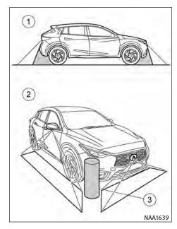
There are some areas where the system will not show objects and the system does not warn of moving objects. When in the front or the rear view display, an object below the bumper or on the ground may not be viewed ①. When in the bird's-eye view, a tall object near the seam ③ of the camera viewing areas will not appear in the monitor ②.
