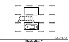
Illustration 2: If the turn signal is then activated, the system chimes (twice) and the BSW indicator light flashes. The BSW indicator light continues to flash until the detected vehicles leave the detection zone.
