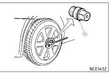
When removing tires, use the lock key provided with your vehicle.
