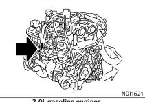
2.0L gasoline engines ENGINE SERIAL NUMBER
