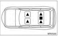
▲ Indicates that the seating position is equipped with a head restraint.
