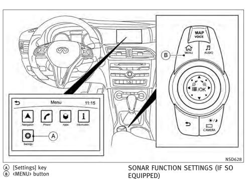
The sonar function settings can be changed using the following procedure.
