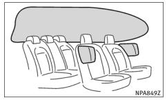
Front seat-mounted side-impact supplemental air bag and window bag/roof-mounted curtain side-impact and rollover supplemental air bag systems
