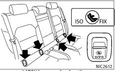
LATCH lower anchor locations LATCH lower anchor location
