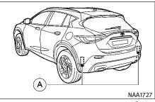
The BSW system uses radar sensors A installed near the rear bumper to detect other vehicles beside your vehicle in an adjacent lane.
