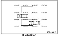
**Illustration 1:** If the radar sensors detect a vehicle in the detection zone, the BSW indicator light (1)located by the outside mirrors illumi-
