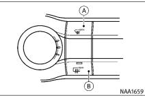
The windshield de-icer switch (defogger switch) A operates when the ignition switch is in the ON position.
