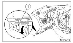
2. Pull the hood lock release lever ①, located below the instrument panel on the driver's side; the hood will spring up slightly.
