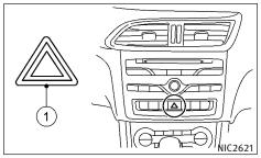
The hazard warning flasher switch (1) operates regardless of the ignition switch position except when the battery is discharged.
