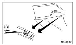
If you wax the surface of the engine hood, be careful not to let wax get into the washer nozzle (a). This may cause clogging or improper wind-shield washer operation. If wax gets into the nozzle, remove it with a needle or small pin (B).
