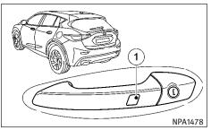
Touch recessed sensor surface (1) on the door handle until the side windows are fully closed.
