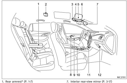
10. Front cup holders (P. 2-79) 11. Air conditioner controls (P. 4-42) 12. Glove box/storage (P. 2-78)
