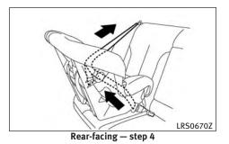
4. Allow the seat belt to retract. Pull up on the shoulder belt to remove any slack in the belt.
