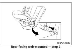
2. Secure the child restraint anchor attachments to the LATCH lower anchors. Check to make sure the LATCH attachment is properly attached to the lower anchors.
