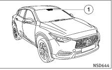
The LDW system uses a camera (1) installed behind the windshield to monitor the lane markers of your traveling lane.
