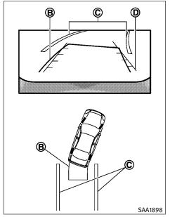
Slowly back up the vehicle adjusting the steering wheel so that the predicted course lines (B) enter the parking space (C).
