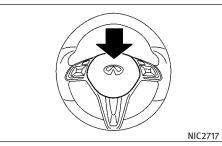
To sound the horn, push the center pad area of the steering wheel.
