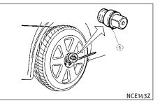
4. Loosen each wheel bolt by one or two turns counterclockwise with the wheel wrench.
