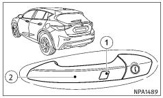
To unlock the vehicle: touch the inner surface of the door handle.
