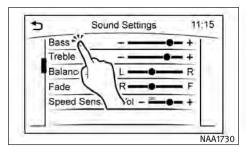
Touch adjustment keys, such as [+]/[-], [L]/[R], etc., to adjust each item. Each time a key is touched, the indicator moves along the bar.
