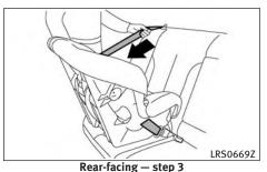
3. Pull the shoulder belt until the belt is fully extended. At this time, the seat belt retractor is in the ALR mode (child restraint mode). It reverts to the ELR mode when the seat belt is fully retracted.
