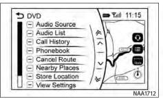
While the current vehicle location is displayed on the map, push  $\langle i i i i i \rangle / OK \rangle$  on the INFINITI controller to display the shortcut menu on the display.
