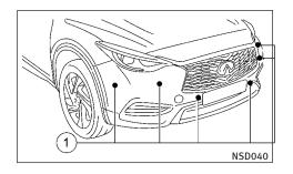
The parking sensor system is an electronic parking aid with ultrasonic sensors. The parking sensor system indicates audibly the distance between your vehicle and an object. It monitors the area around your vehicle using sensors in the front and rear bumper. Possible sensor configurations include a 4 sensor, 10 sensor or 12 sensor configuration.
