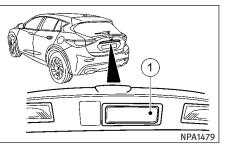
**To unlock the lift gate**: press the lift gate switch ①.
