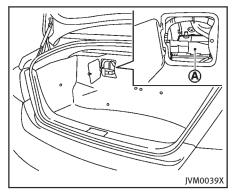
The 12-volt battery  $(\mbox{\textbf{A}})$  is located on the left hand side of the trunk behind an access panel.
