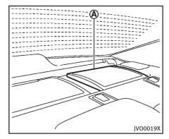
An air vent (A) is located on the rear parcel shelf to cool the Li-ion battery. If the vent is covered, the battery will overheat resulting in reduced output performance of the hybrid system. See "Lithium-ion (Li-ion) battery air vent" (P.7-5).
