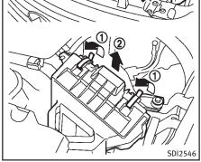
**VQ35HR engine** Remove the retainers ① as illustrated and pull out the filter element ②.
