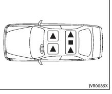
The illustration shows the seating positions equipped with head restraint/head-rest.
