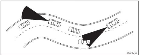
When driving on some roads, such as winding, hilly, curved, narrow roads, or roads which are under construction, the sensor may detect vehicles in a different lane, or may temporarily not detect a vehicle traveling ahead. This may cause the system to work inappropriately.
