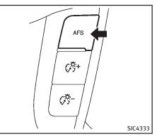
To turn the AFS off, push the AFS switch. (The AFS OFF indicator light will illuminate.) Push the switch again to turn the system on again.
