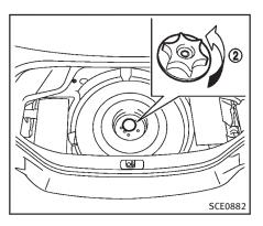
Getting the spare tire and tools Raise the trunk floor cover (1) using the tab (A).
