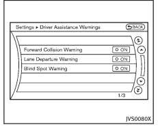
3. Highlight the "Forward Collision Warning" key, select ON (enabled) or OFF (disabled) and push the ENTER (2) button.
