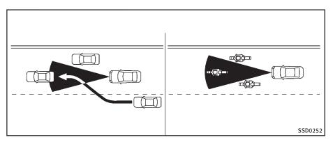
The detection zone of the sensor is limited. A vehicle ahead must be in the detection zone for the system to operate.
