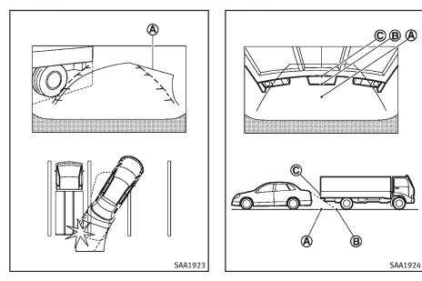
may hit the object when backing up to the position (A) if the object projects over the actual backing up course.
