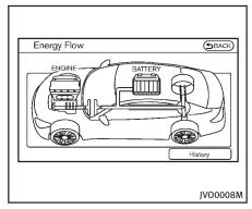
This is an example of the Energy Flow display. The Energy Flow display changes, depending on the following operating conditions. The graphic indicates the amount of power in the Li-ion battery.
