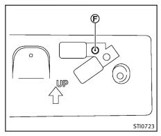
Mark the center of the hole  $(\mathbf{F})$  on both sides with a felt-tip pen. Remove the bracket from the bumper, and then open 0.79 in (20 mm) diameter holes on the bumper using the marks  $(\mathbf{F})$  as a center.
