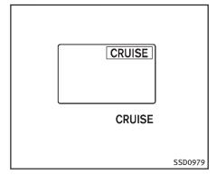
If it is not possible to set the system or the indicator stays on, it may indicate that the ICC system is malfunctioning. Although the vehicle is still driveable under normal conditions, have the vehicle checked at an INFINITI retailer.
