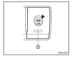
The warning systems switch is used to turn on and off the warning systems (Forward Collision Warning (FCW), Lane Departure Warning (LDW) and Blind Spot Warning (BSW) systems) that are activated using the settings menu on the center display.
