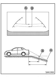
is the place (B). Note that any object on the hill is closer than it appears on the monitor.
