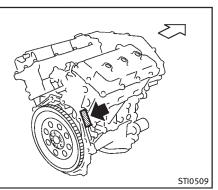
VQ35HR engine ENGINE SERIAL NUMBER
