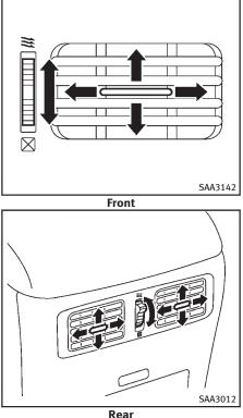
Open or close, and adjust the air flow direction of ventilators.
