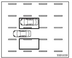
**Illustration 11 – Entering from the side** Illustration 11: If the BSI system is on and your vehicle approaches the lane marker while another vehicle is in the detection zone, the BSW/BSI indicator light flashes and a chime will sound three times. Then, the BSI system slightly applies the brakes on the appropriate side to help return the vehicle back to the center of the driving lane.
