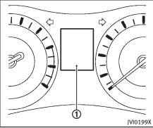
The dot matrix liquid crystal display ① is located between the tachometer and the speedometer, and it displays the automatic transmission position indicator, the cruise control, the Intelligent Cruise Control (ICC) system (if so equipped), the Distance Assist (DCA) system (if so equipped) information, the Intelligent Key operation information and other warnings and information.
