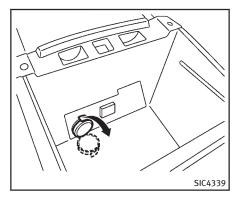
The power outlet is located in the center console.
