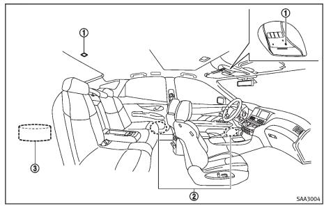
This system uses microphones ① located inside the vehicle to detect engine booming sound. The system then automatically produces a muted engine booming sound through the speakers ② and woofer ③ (if so equipped) to reduce engine booming sound.
