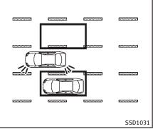
**Illustration 2 – Approaching from behind** Illustration 2: If the driver activates the turn signal, then the BSW/BSI indicator light flashes and a chime will sound twice.
