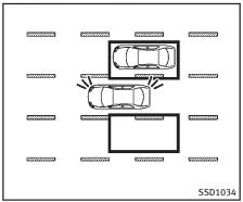
**Illustration 6 – Overtaking another vehicle** Illustration 6: If the driver activates the turn signal while another vehicle is in the detection zone, then the BSW/BSI indicator light flashes and a chime will sound twice.
