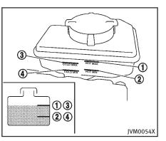
Check the fluid level in the reservoir.
