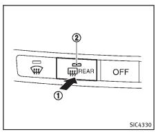
To defog/defrost the rear window glass and outside mirrors, start the hybrid system and push the switch ① on. The indicator light ② will come on. Push the switch again to turn the defroster off.
