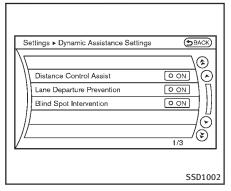
3. Highlight the "Distance Control Assist" key, select ON (enabled) or OFF (disabled) and push the ENTER (2) button.
