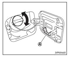
To remove the fuel-filler cap:
