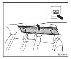
The rear sunshade operates when the power ignition is in the ON position.
