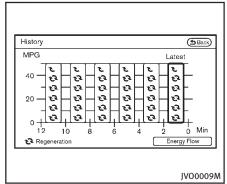
The Fuel Economy History can be displayed on the navigation system monitor. This displays the vehicle's average fuel consumption and regenerative electric power at 2 minute intervals.
