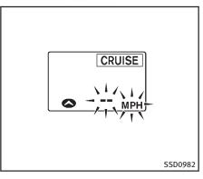
**To set cruising speed,** accelerate your vehicle to the desired speed, push the COAST/SET switch and release it. (Vehicle ahead detection indicator, set distance indicator and set vehicle speed indicator come on.) Take your foot off the accelerator pedal. Your vehicle will maintain the set speed.
