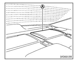
LITHIUM-ION (Li-ion) BATTERY AIR VENT
