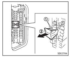
Extended storage fuse switch (if so equipped)
