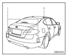
The BSW system uses radar sensors (1) installed near the rear bumper to detect other vehicles beside your vehicle in an adjacent lane. In addition to the radar sensors, the BSI system uses a camera (2) installed behind the windshield to monitor the lane markers of your traveling lane.
