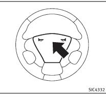
To sound the horn, push the center pad area of the steering wheel.
