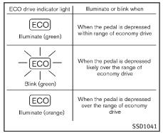
When the ECO drive indicator illuminates in green, the accelerator reaction force is normal. When the ECO drive indicator light
