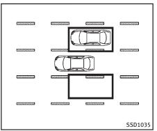
**Illustration 7 – Overtaking another vehicle** Illustration 7: If the BSI system is on and your vehicle approaches a lane marker while another vehicle is in the detection zone, the BSW/BSI indicator light flashes and a chime will sound three times. Then, the BSI system slightly applies the brakes on the appropriate side to help return the vehicle back to the center of the driving lane.
