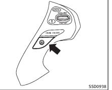
**Dynamic driver assistance switch** The LDP system turns on when the dynamic driver assistance switch on the steering wheel is pushed when the "Lane Departure Prevention" is enabled in the settings menu on the center display. The LDW light (green) on the instrument panel illuminates when the LDP system is turned on.
