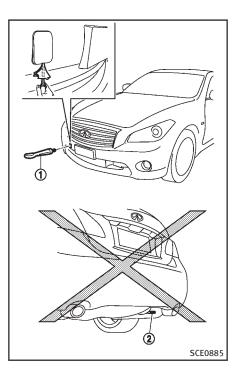
VEHICLE RECOVERY (freeing a stuck vehicle)
