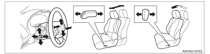
4. Remove front seat head restraint (if necessary).
