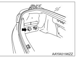
9. Disconnect negative (-) battery cable and cover it with insulated tape.
