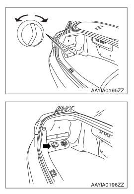
7. Disconnect negative (-) battery cable and cover it with insulated tape.
