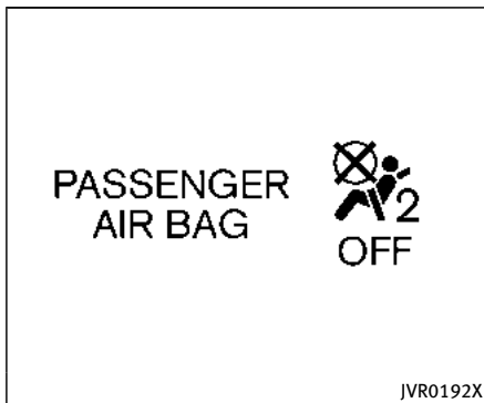
Front passenger air bag and status light
