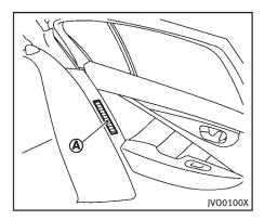
LITHIUM-ION (Li-ion) BATTERY AND DC/DC CONVERTER AIR VENT
