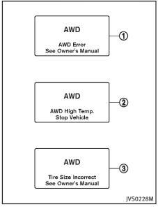
If the "AWD Error" warning ① appears, there may be a malfunction in the Intelligent AWD system. Reduce vehicle speed and have your vehicle checked by an INFINITI retailer as soon as possible.
