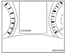
Five driving modes can be selected by using the INFINITI Drive Mode Selector (PERSONAL, SPORT, STANDARD, ECO and SNOW).
