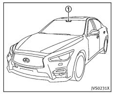
Active Lane Control slightly corrects front tire angles and steering wheel torque to help reduce the difference between the vehicle's direction and the lane direction (2) which is detected by using the camera unit (1) located above the inside mirror.
