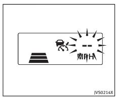
When the SET/COAST (-) switch is pushed under the following conditions, the system cannot be set and the ICC indicators will blink for approximately 2 seconds:
