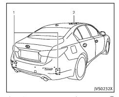
The BSW system uses radar sensors (1) installed near the rear bumper to detect other vehicles in an adjacent lane. In addition to the radar sensors, the BSI system uses a camera (2) installed behind the windshield to monitor the lane markers of your traveling lane.
