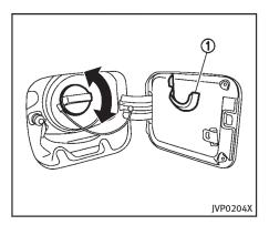
To remove the fuel-filler cap:
