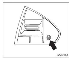
Dynamic driver assistance switch Active Lane Control turns on when the dynamic driver assistance switch on the steering wheel is pushed and [Active lane control] and [Lane Departure Prevention] are enabled in the settings menu on the lower display. See "How to enable/disable the LDP system" (P.5-35).
