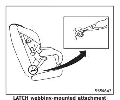
Installing child restraint LATCH
