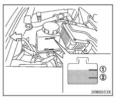
Check the fluid level in the reservoir. If the fluid is below the MIN line (2) or the brake warning light comes on, add Genuine NISSAN Super Heavy Duty Brake Fluid or equivalent DOT 3 fluid up to the MAX line (1). If fluid must be added frequently, the system should be checked by an INFINITI retailer.
