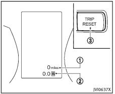
Odometer/twin trip odometer
