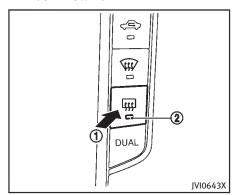
To defog/defrost the rear window glass and outside mirrors, start the INFINITI Direct Response Hybrid® System and push the switch ① on. The indicator light ② will come on. Push the switch again to turn the defroster off.
