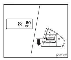
To set cruising speed, accelerate your vehicle to the desired speed, push the SET/COAST (-) switch and release it. (The color of the cruise indicator changes to green and set vehicle speed indicator comes on.) Take your foot off the accelerator pedal. Your vehicle will maintain the set speed.
