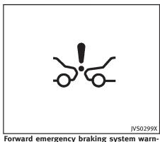
orward emergency braking system warning light (orange)
