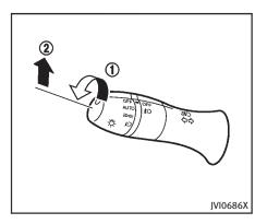
To turn off the high beam assist system, turn the headlight switch to the position or select the low beam position by placing the lever in the neutral position.
