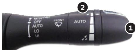
Move the lever ① up or down to one of the following positions to operate the windshield wipers:
