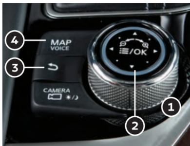
Use the Infiniti controller (1) and **OK** button (2) to navigate through the upper display screens.
