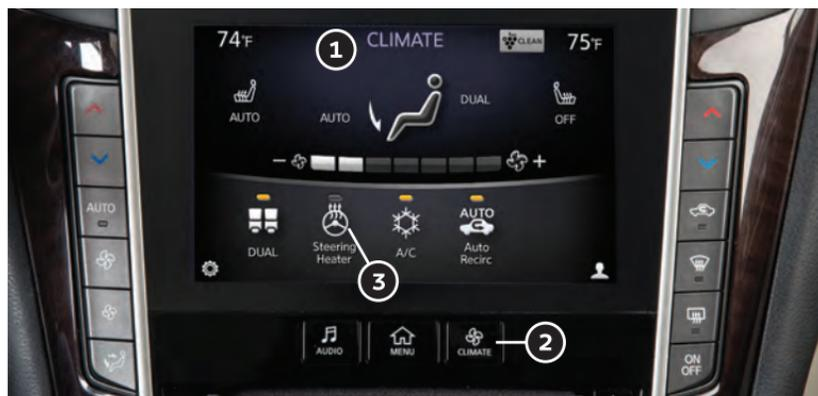
The climate controls can be adjusted using the buttons on either side of the lower display or through the "CLIMATE" screen (1) on the lower display.
