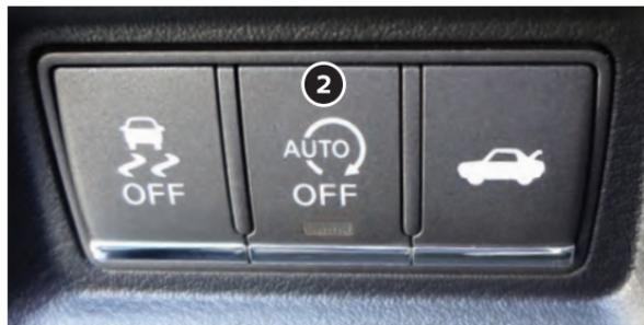
The ISS activates to prevent unnecessary fuel consumption, exhaust emissions and noise.
