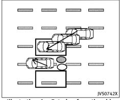
Illustration 6 - Entering from the side Illustration 6: If the driver activates the turn signal, then the system chimes (twice) and the side indicator light flashes.
