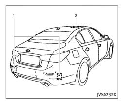
The BSI system uses radar sensors (1) installed near the rear bumper to detect other vehicles in an adjacent lane. In addition to the radar sensors, the BSI system uses a camera (2) installed behind the windshield to monitor the lane markers of your traveling lane.
