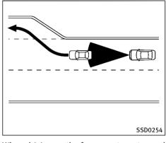
When driving on some roads, such as winding, hilly, curved, narrow roads, or roads which are under construction, the radar sensor may detect vehicles in a different lane, or may temporarily not detect a vehicle traveling ahead. This may cause the ICC system to decelerate or accelerate the vehicle.
