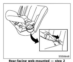
2. Secure the child restraint anchor attachments to the LATCH lower anchors. Check to make sure the LATCH attachment is properly attached to the lower anchors.
