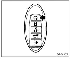
The remote engine start  $\Omega$  button is on the Intelligent Key if the vehicle has remote engine start function. This function allows the engine to start from outside the vehicle.
