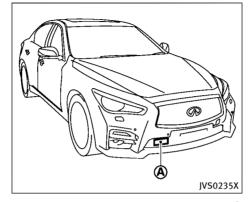
The PFCW system uses a radar sensor (A) located behind the lower grille of the front bumper to measure the distance to a second vehicle ahead in the same lane.
