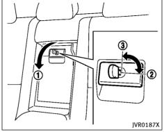
key cylinder before opening or closing the lid. Otherwise the lid and the rear armrest may be damaged.
