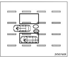
Illustration 3 - Approaching from behind Illustration 3: If the BSI system is on and your vehicle is approaching a lane marker and a vehicle is in the detection zone, the system chimes a sound (three times) and the side indicator light flashes. The BSI system activates to help return the vehicle back to the center of the driving lane.
