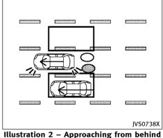
Illustration 2: If the driver activates the turn signal then the system chimes a sound (twice) and the side indicator light flashes.
