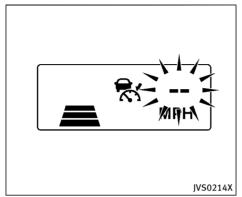
When the SET/COAST (-) switch is pushed under the following conditions, the system cannot be set and the ICC indicators will blink for approximately 2 seconds:
