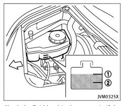
Check the fluid level in the reservoir. If the fluid is below the MIN line (2) or the brake warning light comes on, add Genuine NISSAN Super Heavy Duty Brake Fluid or equivalent DOT 3 fluid up to the MAX line (1). If fluid must be added frequently, the system should be checked. It is recommended you visit an INFINITI retailer for this service.
