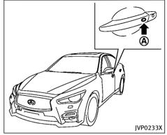
When you carry the Intelligent Key with you, you can lock all doors by pushing the door handle request switch (A) (driver's or front passenger's) within the range of operation.
