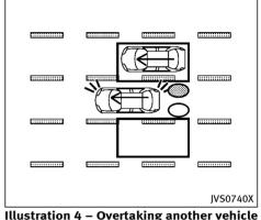
Illustration 4 – Overtaking another vehicle Illustration 4: If the driver activates the turn signal while another vehicle is in the detection zone, then the system chimes (twice) and the side indicator light flashes.
