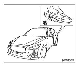
You can also unlock the corresponding door by touching the one touch unlock sensor (B) (driver's or front passenger's) within the range of operation, and can unlock the other doors using the door handle request switch (A).
