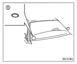
Be sure not to put anything on top of the photo sensor (1) located on the top of the instrument panel. The photo sensor controls the autolight; if it is covered, the photo sensor reacts as if it is dark and the headlights will illuminate.
