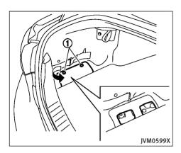
AUXILIARY BATTERY LOCATION (for 2.0L turbo gasoline engine models)
