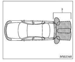
The radar sensors (1) detect an approaching vehicle from up to approximately 49 ft (15 m) away. The sonar sensors (2) detect stationary objects behind the vehicle up to approximately 4.9 ft (1.5 m). Refer to the illustration for approximate zone coverage areas (3).
