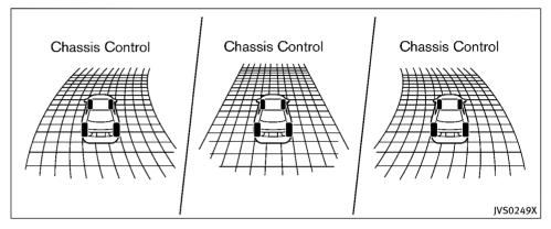
When the active trace control is operated and the "Chassis Control" mode is selected in the trip computer, the active trace control graphics are shown in the vehicle information display. (See "Trip computer" (P.2-31).)
