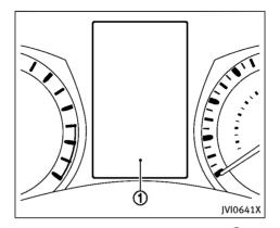
The vehicle information display ① is located between the tachometer and the speedometer, and it displays the warnings and information. The following items are also displayed if the vehicle is equipped with them:
