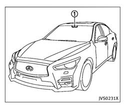
The LDW and LDP systems use a camera ① installed behind the windshield to monitor the lane markers of your traveling lane.
