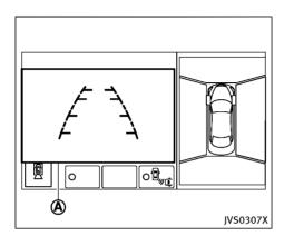
If an approaching vehicle or object behind the vehicle is detected when your vehicle is backing up, red frame (A) will appear on the upper display and the system will chime three times. Then, the brakes will be applied momentarily. After the automatic brake application, the driver must depress the brake pedal to maintain brake pressure.
