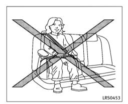
Make sure the child's head will be properly supported by the booster seat or vehicle seat. The seatback must be at or above the center of the child's ears. For example, if a low back booster seat is chosen, the vehicle seatback must be at or above the center of the child's ears. If the seatback is lower than the center of the child's ears, a high back booster seat (2) should be used.
