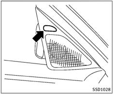
If the radar detects an approaching vehicle from the side, the system chimes a sound (single beep), the side indicator light on the side the vehicle is approaching from flashes and a yellow rectangular frame (A) appears on the upper display.
