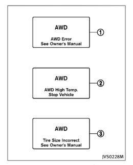
If the "AWD Error" warning ① appears, there may be a malfunction in the Intelligent AWD system. Reduce vehicle speed and it is recommended you have your vehicle checked by an INFINITI retailer as soon as possible.
