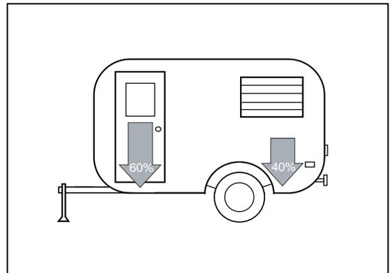
The trailer load should be balanced equally from side-to-side. Unequal side-to-side loading can negatively affect handling and braking. Once in place, all cargo should be firmly secured to prevent shifting. If the load should shift abruptly during braking or cornering, it could quickly affect the handling of your vehicle and cause a very unsafe situation.
