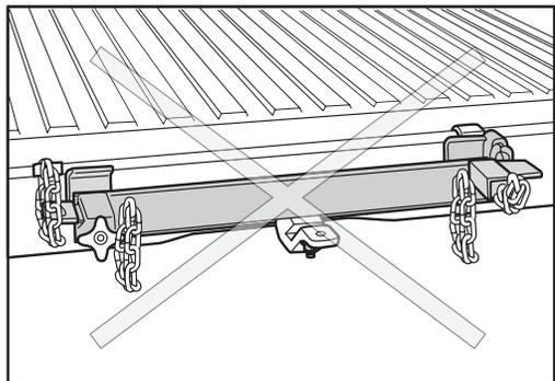
**Weight-Distributing Hitch System** – This type of system uses a “load-leveling” or “equalizing” hitch. The weight-distributing feature helps shift the trailer tongue weight to all trailer tires and the tow vehicle front tires.
