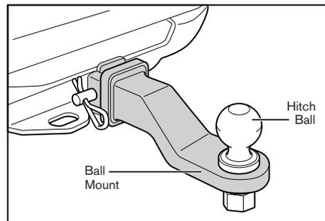
Like ball mounts, hitch balls are available in a number of weight capacities and sizes. Always make sure the hitch ball selected has the proper shank diameter and weight rating for the ball mount as well as the coupler on your trailer. Using a 1<sup>7</sup>/<sub>8</sub>” hitch ball in a 2” coupler, for example, could result in the trailer separating from the tow vehicle.
