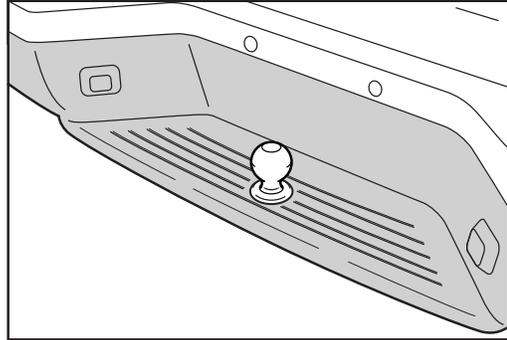
**Receiver Hitch** – A receiver hitch is bolted directly to the vehicle structure for added strength and durability. Infiniti bolt-on receiver hitches are designed specifically for Infiniti vehicles and include the necessary reinforcements, with ample clearance around bumpers, frame members, etc. These hitches allow for the removal of the ball mount when not towing.
