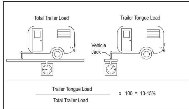
For proper handling, you must keep the trailer tongue load between 10-15% of the actual trailer weight, within the limits of the maximum trailer tongue load allowable. For example, to determine the proper trailer tongue load for a 1,500-lb. trailer, multiply the weight of 1,500 lbs. by 10% to arrive at a figure of 150 lbs.
