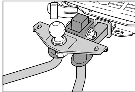
**NOTE** – A weight-distributing hitch system may affect the operation of trailer surge brakes. If you are considering use of a weight-distributing hitch system with a surge brake-equipped trailer, check with the surge brake, hitch, or trailer manufacturer to determine if and how this can be done. Follow the instructions provided by the manufacturer for installing and using the weight-distributing hitch system.
